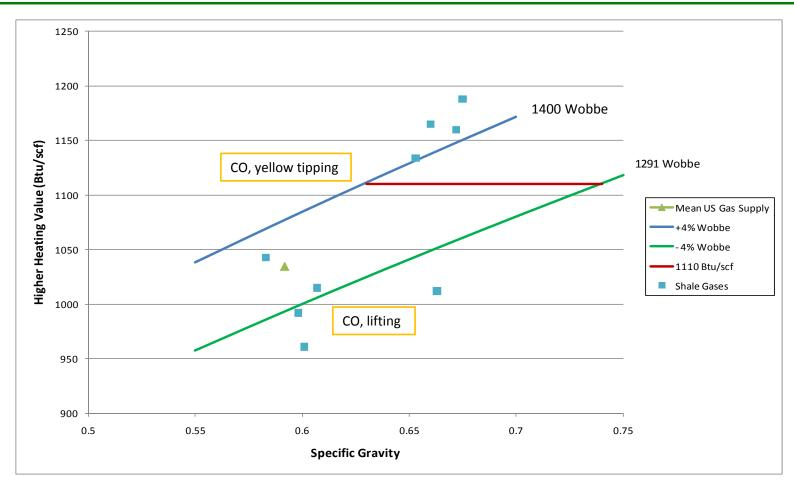
Processing to remove some ethane + propane or carbon dioxide + nitrogen or, when feasible, blending with other natural gases can shift shale gases into the "range of acceptability".
